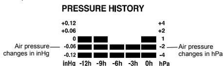
The horizontal axis represents the last 12 hours air pressure recording (-12, -9, -6, -3 and 0 hour). The bars are plotted at each of the 5 steps and give the trend over the recorded period. The scale on the right compares the result. The "0" in the middle of this scale determines the current air pressure.
