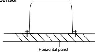
For best results, the rain sensor should be securely mounted onto a horizontal surface about 39.37" (1 meter) above the ground (or higher) and in an open area away from trees or other coverings where rainfall may be reduced causing inaccurate readings.
