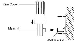
An ideal mounting place for the thermo-hygro sensor would be the outer wall beneath the extension of a roof, as this will protect the sensor from direct sunlight and other extreme weather conditions.
