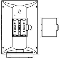
The Weather Center works with 3 x AA, IEC LR6, 1.5V Alkaline batteries. When the batteries need to be replaced, the low battery symbol will appear on the LCD. To install and replace the batteries, please follow the steps below:
