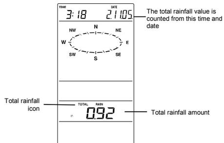
To reset the rainfall reading, press the + key once when the Rainfall value and "Reset" icon is shown. Then the total rainfall amount will be reset to 0, and the time updated to current time.
