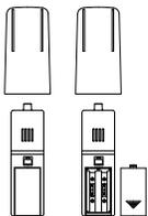
The outdoor Thermo-hygro sensor works with 2 x AA, IEC LR6 1.5V Alkaline batteries. To install and replace the batteries, please follow the steps below:
