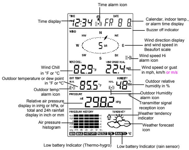
\* When the signal from the transmitter/ or Rain sensor is successfully received by the Weather Station, this icon will be switched on. (If not successful, the icon will not be shown on the LCD). User can therefore easily see whether the last reception was successful ("ON" icon) or not ("OFF" icon). On the other hand, the short blinking of the icon shows that a reception is being done at that time.
