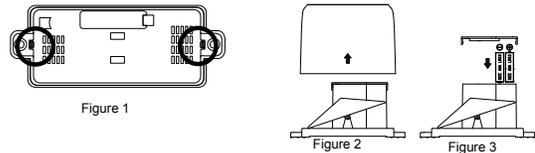
The rain sensor works with 2 x AAA, IEC LR3, 1.5V Alkaline batteries. To install and replace the batteries, please follow the steps below:
